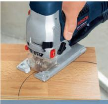
The Special for Laminate jigsaw blades are also available for precision curved cuts.
