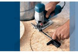
At the building site, use the Progressor for Wood and Metal T 345 XF to cut through wood (even if it contains nails), metal plate, pipes and aluminium profiles.
